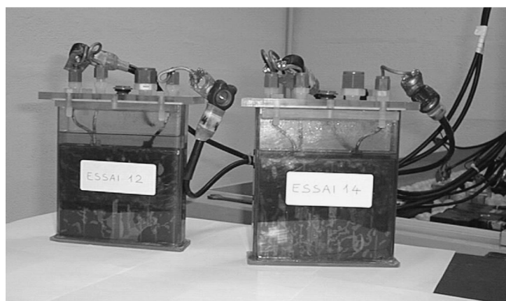
Fig. 1. Cells for tests of additives in real electrode scale.
